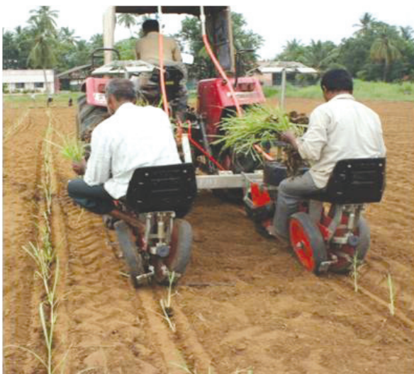
Fig. 1. Budchip seedling transplanter in operation
