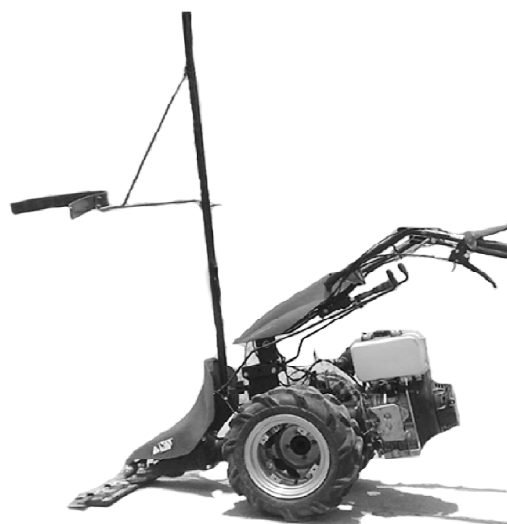
Fig.1. Sugarcane harvester machine fitted with developed guide bar
