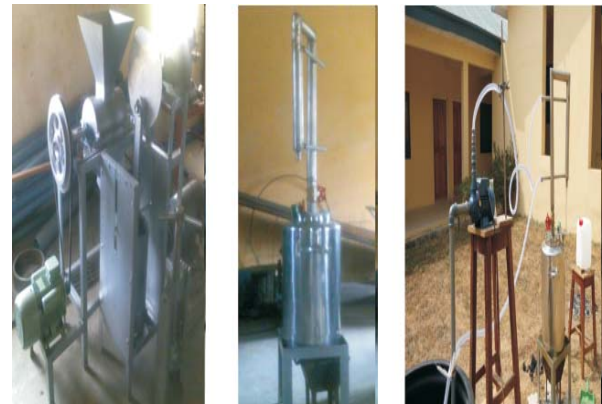
Fig. 1. View of sugarcane juice extractor (left), fermenter (middle) and distillation unit (right)
