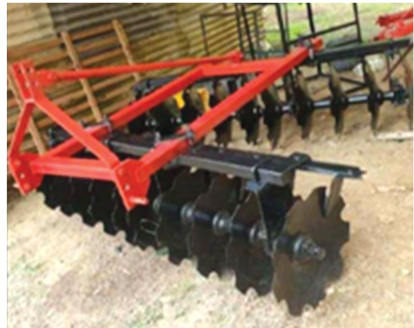
Figure 3. A disc plough (left top), a spike harrow (left bottom) and a disc harrow(top)
