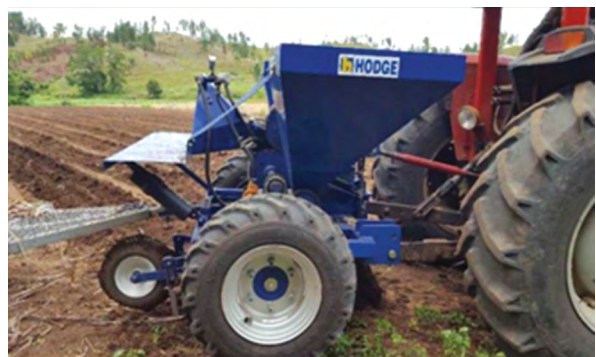
Figure 6. Whole stalk cane planter machine
